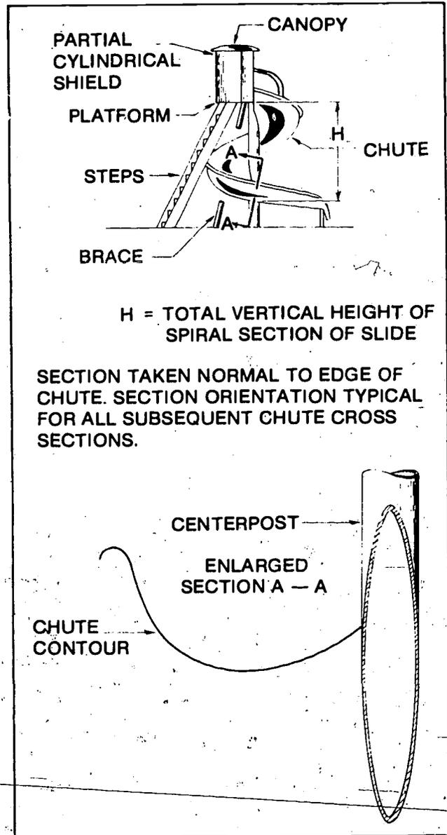
H = TOTAL VERTICAL HEIGHT OF SPIRAL SECTION OF SLIDE
