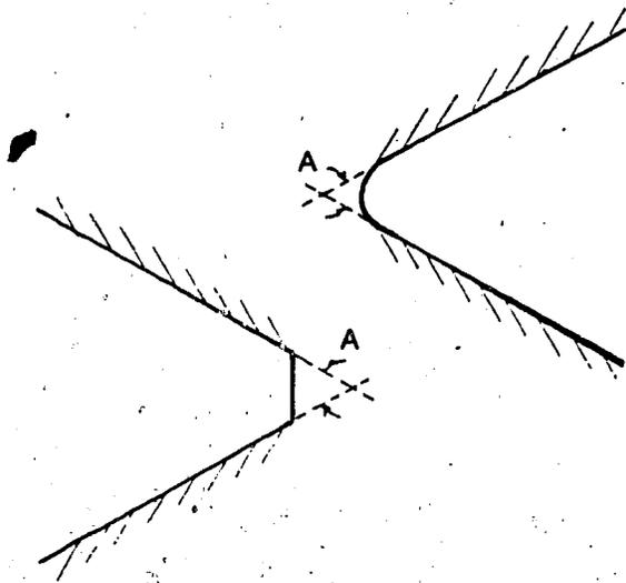
**FIGURE 13 - PROJECTED LINES OF INTERSECTION FOR DETERMINING ANGLE A**
