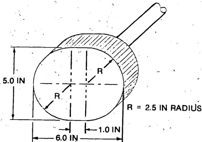
**FIGURE 14 - PROBE FOR DETERMINING ACCESSIBLE OPENINGS**
