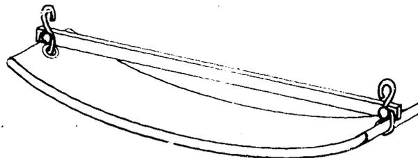
**FIGURE 10a - BRACE FOR FLEXIBLE SEATS**
