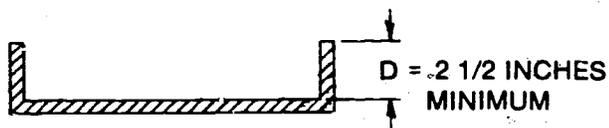
**FIGURE 19 - SLIDE CROSS SECTION**
