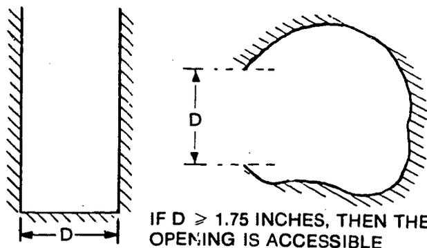
**FIGURE 15 - PARTIALLY BOUNDED OPENINGS**
