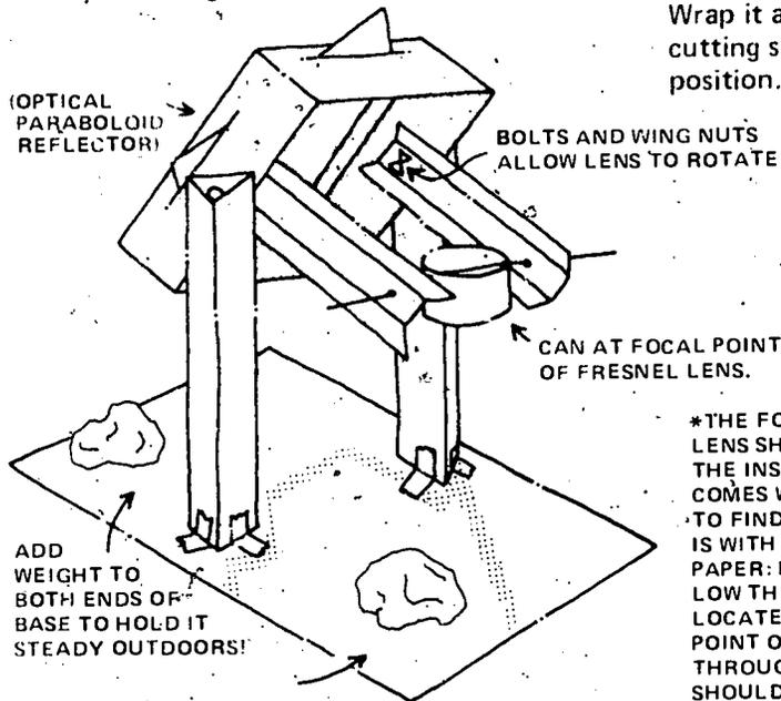
\*THE FOCAL LENGTH OF YOUR LENS SHOULD BE LISTED ON THE INSTRUCTION SHEET THAT COMES WITH IT. ANOTHER WAY TO FIND THE FOCAL LENGTH IS WITH A SHEET OF WHITE PAPER: MOVE THE PAPER BELOW THE LENS UNTIL YOU LOCATE THE SMALLEST PIN-POINT OF LIGHT COMING THROUGH IT. THE PAPER SHOULD IGNITE AND BURN.
