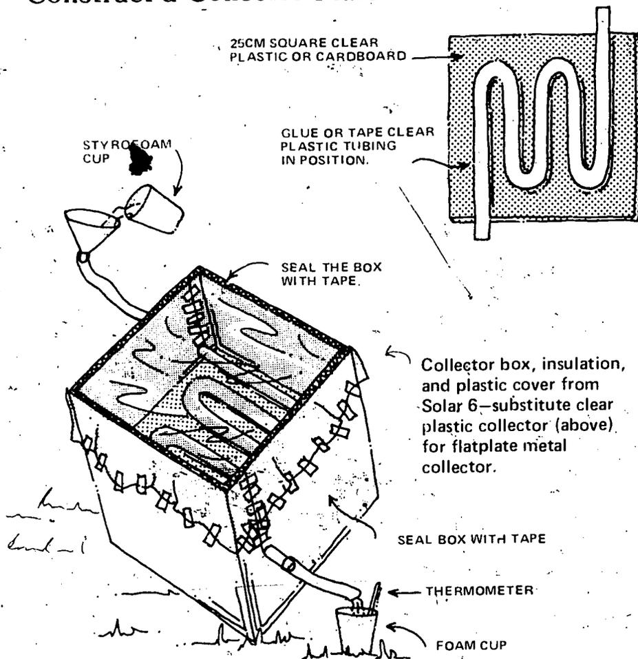
Put the clear plastic collector plate in the box from Activity 6, and face the collector directly into the sun.
