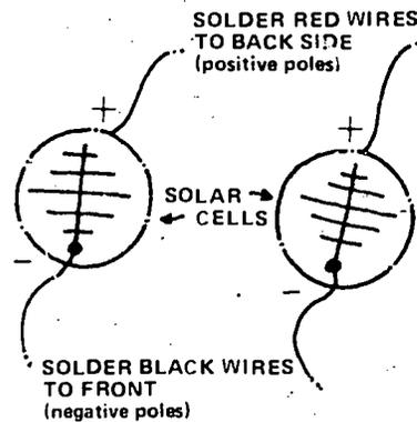
Place the solar cells in full sun and measure milliamps and volts.
