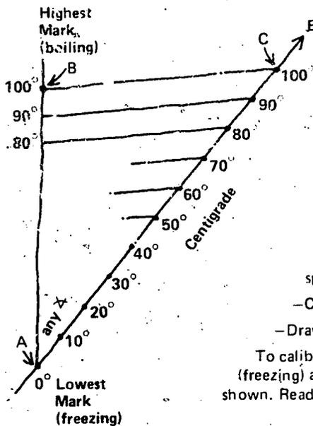
Divide the space between the boiling and freezing marks on your thermometer into 10 equal spaces—an easy way to do this follows:
