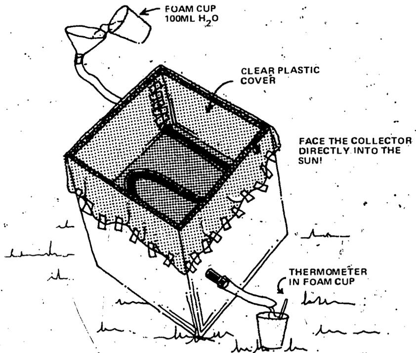
Check the box to be sure all cracks and holes are tightly sealed!
