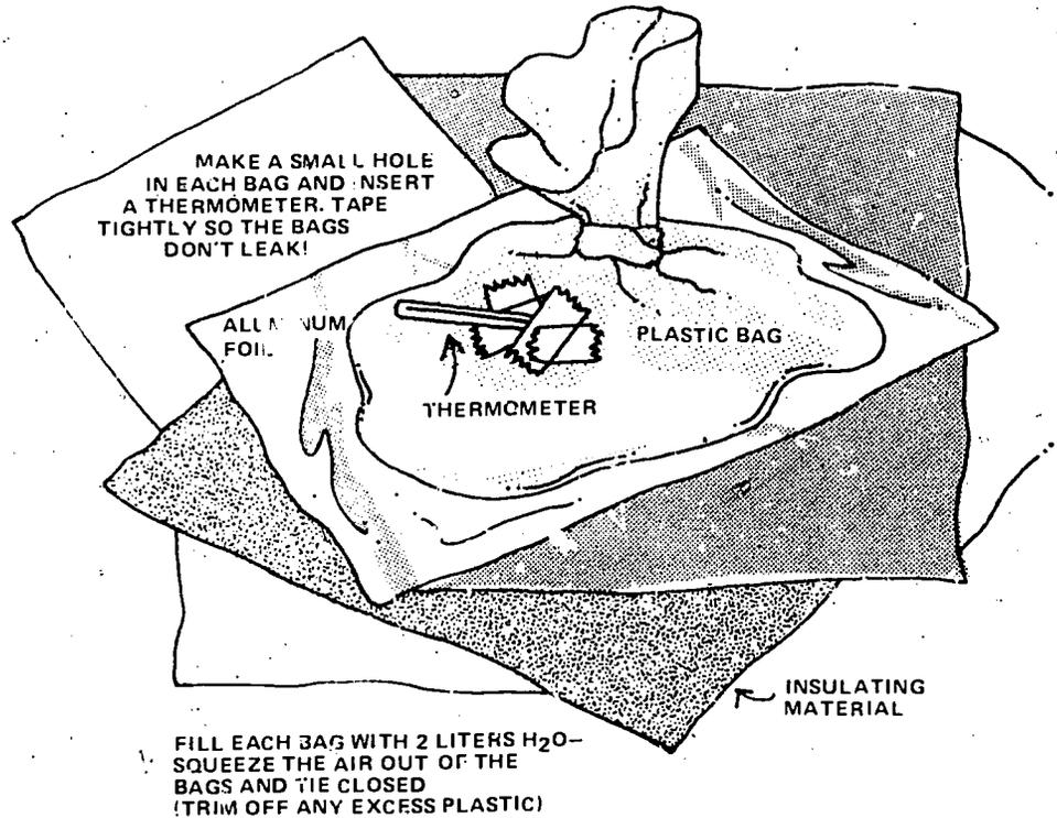
Record the temperatures of the 3 collectors, and place the collectors on the foil in the sun.
