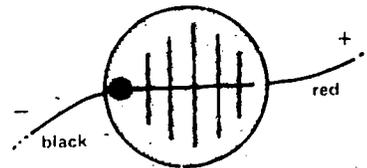
Remove the battery and connect a photocell to the sound generator.
