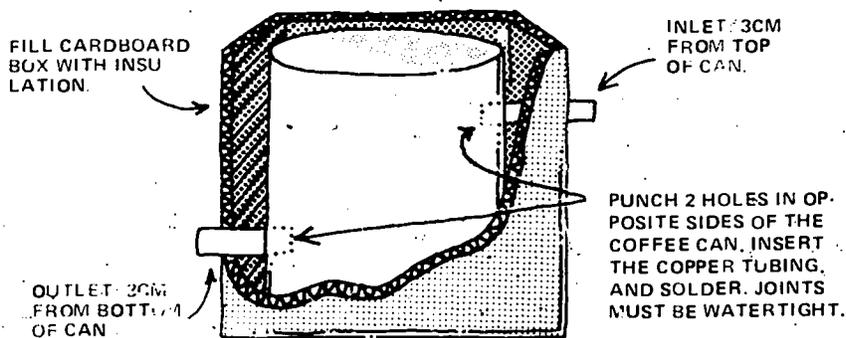
BOTTOM OF CAN SHOULD BE ABOVE TOP OF SOLAR COLLECTOR.
