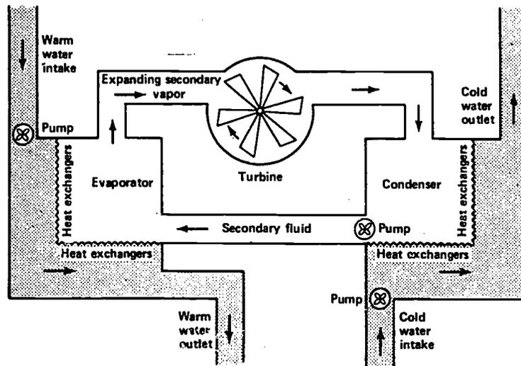
Figure 17 Diagram of a closed cycle ocean thermal power plant.
