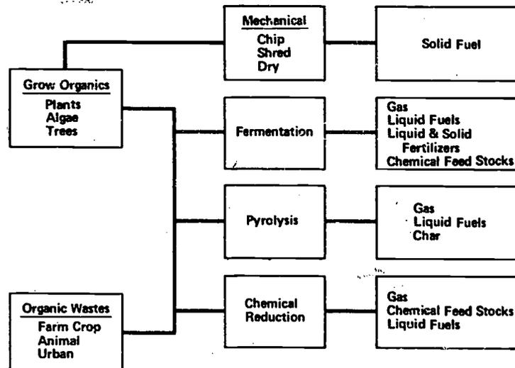
**Figure 18** *Various methods of producing different kinds of fuels from solar energy.*
