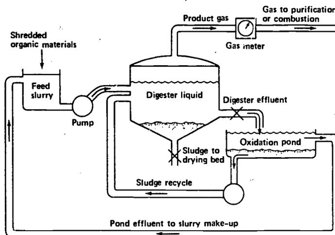
**Figure 19** *Concept of a unit for continuous conversion of organic material to methane by anaerobic fermentation (without oxygen).*
