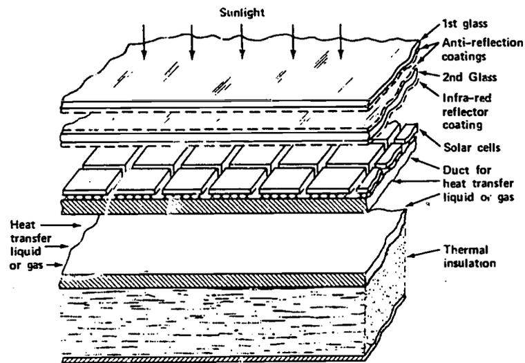
Figure 15 Combination collector arrangement to extract both electrical and heat energy from sunlight.
