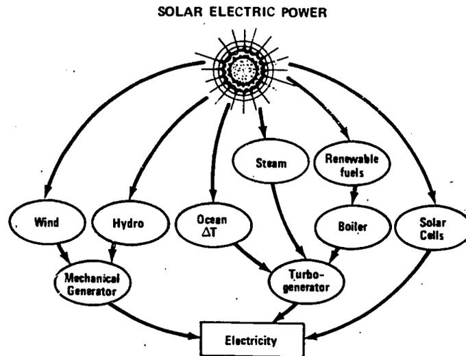
**Figure 10** This diagram shows the various routes by which solar energy can be converted to electricity.
