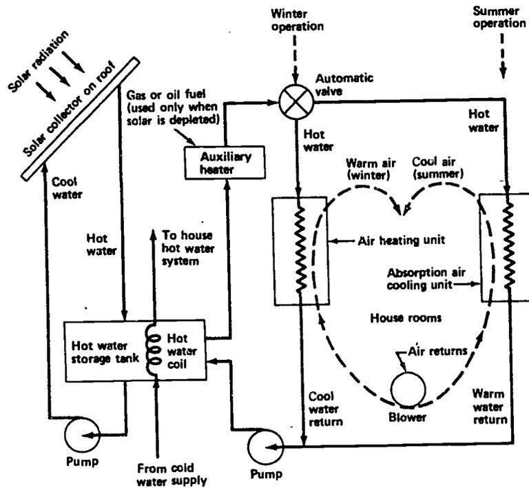
Figure 8 This diagram shows a system that combines residential heating and cooling with solar energy.
