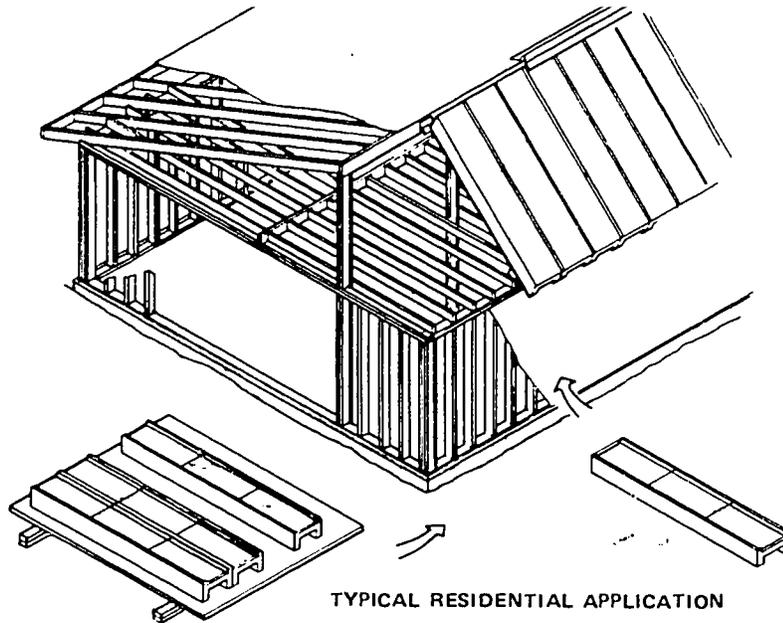
*The flat plate solar collector unit can be architecturally integrated into a building (cutaway view above). The unit is weathertight and insulated. It is easily installed and maintained by building craftsmen.*
