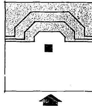
Square plan with parallel walls will create continuous regular sound reflections producing standing waves which may distort the sound.
