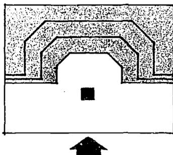
This is preferable to the square plan with respect to the seating arrangement. The acoustics are improved, but the continuous sound reflection still exists to a smaller degree. This can be treated by serrated walls.
