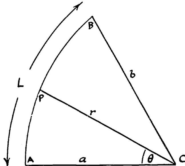
radius  $OP$ , and  $k$  is a constant defining the rate of expansion of the spiral (see Figure 5). The length of the arc  $AB$  of the spiral, when radii  $OA$  and  $OB$  are of lengths  $a$  and  $b$  respectively, is then
