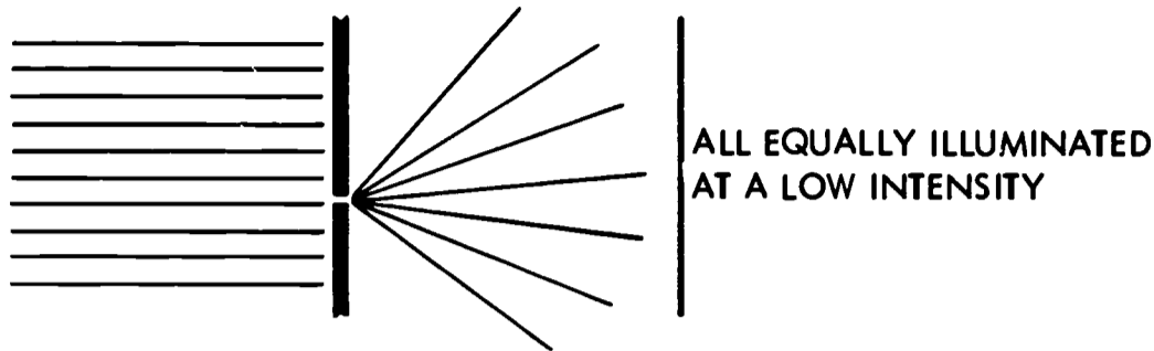
Fig. 2.19 Condition for no shadow: a \ll \lambda . The light passing through the narrow slit
