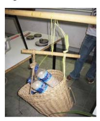
**Figure 4**. Students are testing tensile strength on leaves from different species of palm and of different ages. Weight is added to the basket until breakage occurs, and then the weights at which catastrophic failure are added up. Results are then graphed and compared with the students' predictions.
