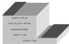
Fig. 2. Structure of the blue LED under study.
