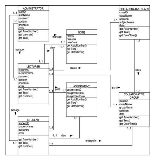
Figure: 3 Class Diagram for OCLS
