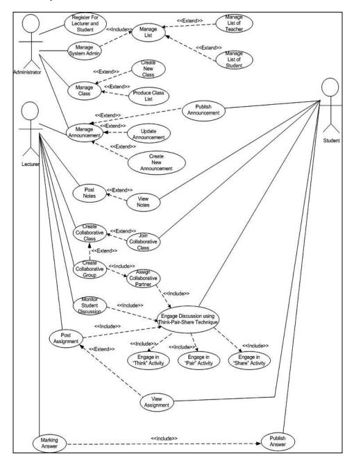
Figure: 2 Use-Case diagram for OCLS
