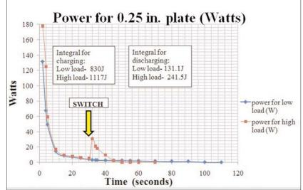
Figure 3 – Scatter plot of calculated power curve for low and high load for 0.25 in. plate
