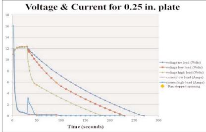
Figure 2 – Scatter plot showing averaged voltage and current values vs. time for all load settings for 0.25 in. plate
