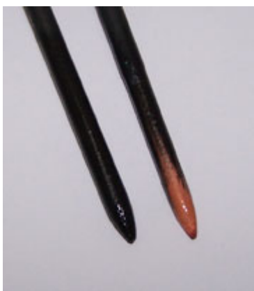
Figure 3. The graphite anode (left) and cathode (right) after being taken out of the solution.
