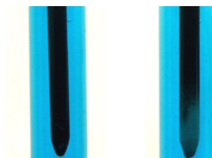
Figure 2. The graphite cathode in the \text{CuSO}_4(\text{aq}) solution before (left) and after (right) passing the current. A whitish-grey cover is noticeable on the lower part of the electrode (right).
