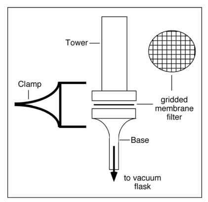
Figure. 1. Schematic view of a Millipore filter apparatus.
