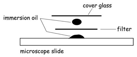
Figure. 3. Preparation the membrane filter for observation.
