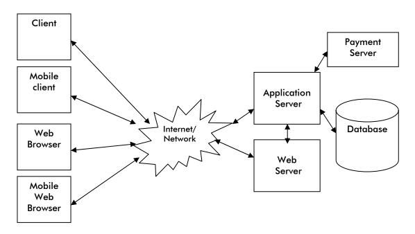
Figure 1. Architecture of a collaborative system
