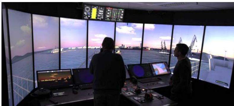
Figure 1. Maritime pilots in training approaching port in a full mission bridge simulator.
