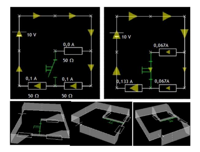
*Figure 3.* Screen Displays of the Simulation Program CLOC (See text). The Separate Window Showing the Circuit in 3D Can Be Rotated continuously.
