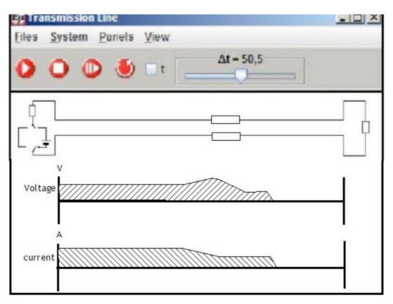
Figure 6. Transition Process for a Serial Circuit (Resistors on Both Lines Plus Load)
