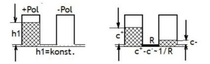
Figure 9. Model for a Battery (Left) and Resistor R with Two Connections (Right)
