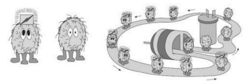
Figure 1. A misleading Model for The Electric Circuit (Electrons with their own driving force (which does not exist of course) are carrying energy from the battery to the motor and return without energy)
