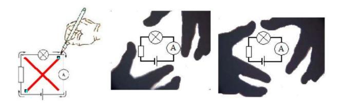
**Figure 4.** Indicating the Movement of Electrons, not Point-By-Point From Minus to Plus (Left) But Collectively as an Interrelated Ring of Electrons
