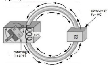
**Figure 8.** Symbolic Representation of an Alternating Voltage Powered Circuit
