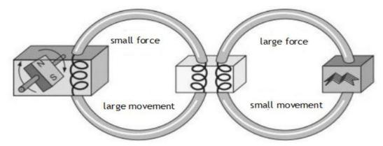
Figure 9. Symbolic Representation of an AC-Current Connected to a Transformer
