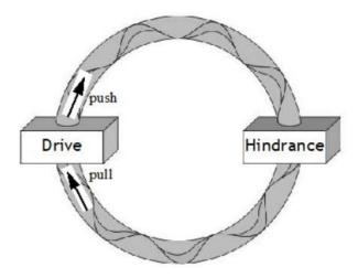
Figure 7. Symbol For an Electric Circuit (Without Branching Points)
