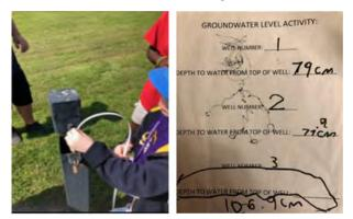
Figure 1: Participant using water level meter to make groundwater level measurement and sample of recorded data
