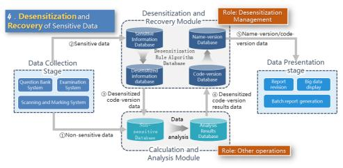
Figure 7. A Schematic Diagram of Data Flow in the Desensitization and Recovery Module.
