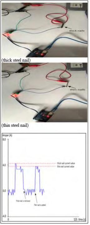
**Figure 6.** Experiment Setup for the Crosssectional Area of the Conductor and the Observation Made on the Serial Plotter
