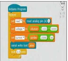
Figure 2. Ready-to-use Code Prepared Using mBlock
