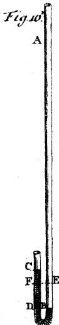
Fig. 7. R. BOYLE, New Experiments Physico-Mechanical , London, 1662; Works , vol.1, End- plate Fig. 16. BOYLE'S J-tube apparatus
