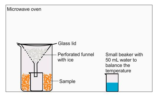
Figure 2. Kitchen microwave extraction setup.
