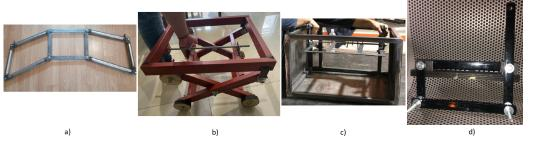
**Figure 5.** The best four prototypes developed in the Regular group. (**a**) Suspension prototype for a retail pushcart, (**b**) workshop table with a lift mechanism, (**c**) grill with a mechanism to select between two levels, (**d**) wiper washer mechanism. In these cases, links were manufactured with steel, and rotation joints were implemented with regular screws.
