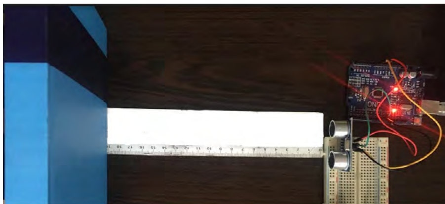
Figure 11: Connection diagram of HC-SR04 with Arduino.
