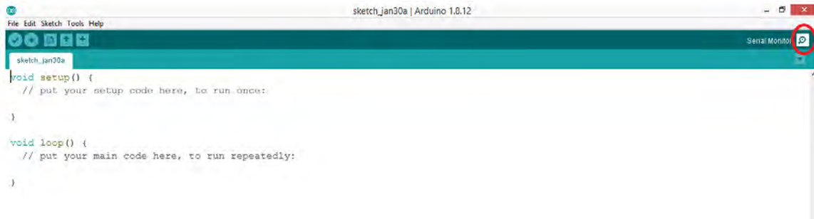
Figure 3: Arduino IDE window. Click the Serial Monitor Icon to open the Serial Monitor.
