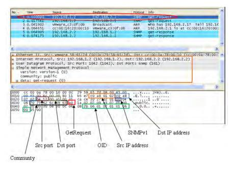
Figure 4. SNMP message analysis using Wireshark.
