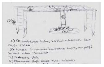
The S9 placed electromagnets connected to a mechanism running on a rail system and stated that the attraction of the electromagnet could be controlled via a remote control system. Moreover, s/he stated that the same apparatus could be made with a non-automatic system.
