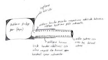
The S17 placed small magnets on a cylindrical metal surface. Metal wastes, from mixed wastes sent to cylindrical metal surface, would be attached to the surface with these magnets and then sent to the collection warehouse. While the student was making the drawing, s/he stated an opinion, "I will benefit from the fields of physics and mathematics, but s/he did not give any details".
