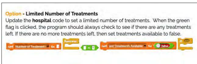
FIGURE 8. Example option of functionality students' can choose to add to their model. In this example, the behavior to be added to the disease model is for hospitals to have a limited number of available treatments.
