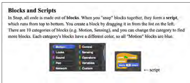
FIGURE 5. In this figure, readers can see how basic elements of the block-based programming are presented and explained in the supplemental materials of the curriculum module to provide scaffolding for students with less familiarity with programming.
