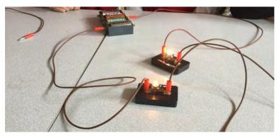
Figure 3. Connecting in series bulbs
