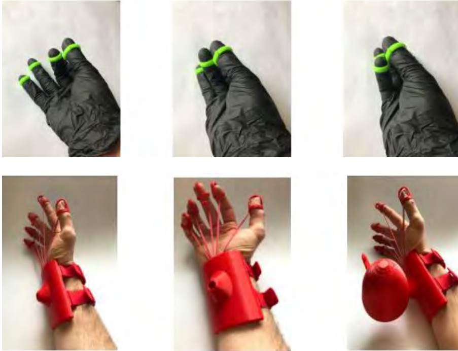
Figure 8: Comparison of low-fidelity prototype versus final result. Note the change in design and prototyping methods to account for functional usability and validation as the project progressed.
