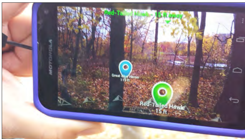
FIGURE 7. The visual display of a location-based hotspot on the augmented reality client-side application using a heads-up display.
