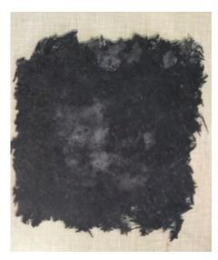
Figure 3. Recycled CFRP sample result from the autoclave curing cycle.
