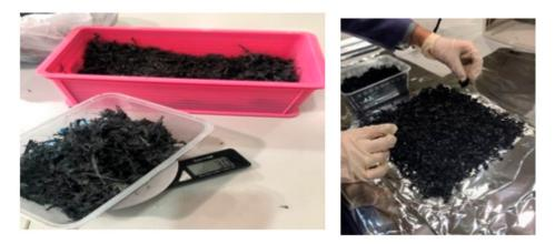
Figure 1. Shredded CFRP preparation for the autoclave process.
