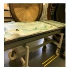
Figure 2. Autoclave to process the waste CFRP under the curing cycle.
