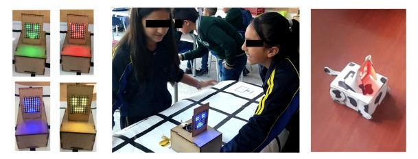
**Figure 3.** Actor robots used in the second experiment. These robots had a screen to enhance the emotional expressiveness of the robots. They also had a speaker for audio playback.
