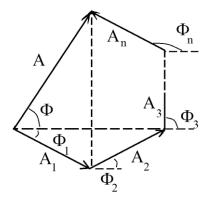
Figure 5. Multipath interference
