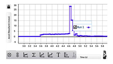
*Figure 8.* The graph of the acceleration in relation to time directly from the screen of an MP using the SPARKvue app
