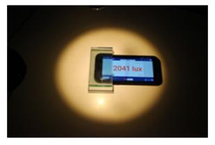
Figure 6. The experimental layout to obtain measurements with MPs equipped with a light sensor
