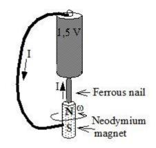
Figure 1. The "simplest" motor
