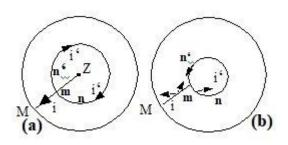
Figure 9. (a) The arrows indicate the tangential microscopic current i' of the magnet and the radial macroscopic current i flowing outside the magnet.
