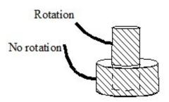
Figure 3. Arrangement for moving the contact point to the outside.
