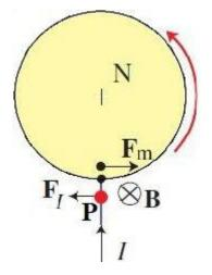
Figure 4. Top view of the magnet indicating the action and reaction forces (see text)
