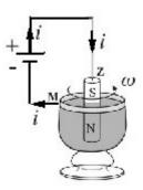
Figure 6. (a) A schematic representation of Ampère's motor
