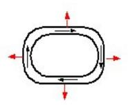
Figure 7. Magnetic forces between oppositely oriented circuit elements
