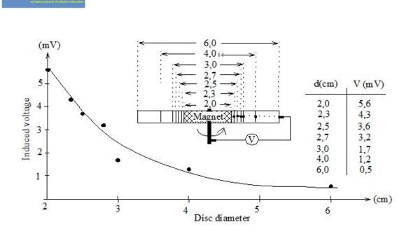
*Figure* 7. *Measurement of the inductance voltage on ring-shaped aluminum discs, which rotate together with a magnet inside around a fixed axis*
