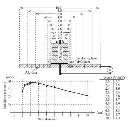
Figure 5. Measurement of the induced voltage for rotating discs of different size
