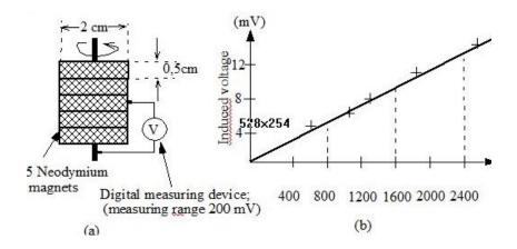
*Figure 3.* (a) Used permanent magnet; (b)  $V_{ind} = f(\omega)$
