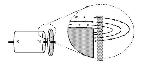
Figure 2. Magnetic lines through an aluminum disc with a slightly larger diameter than the magnet
