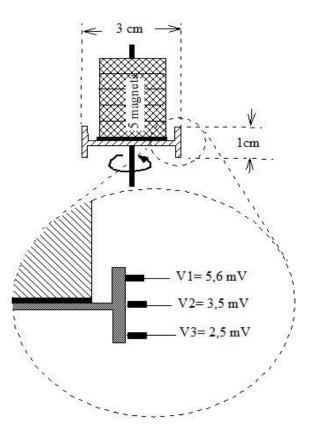
Figure 10. Measurement of the induced voltage on a disc with an enlarged outer surface
