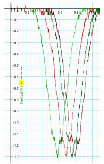
Figure 4. The changes of tension force in four launching.
