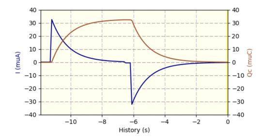
*Figure 1:* Real-time plotted electric charge Q and current I in an RC-circuit acquired with the data logger module in the ADS1115 configuration
