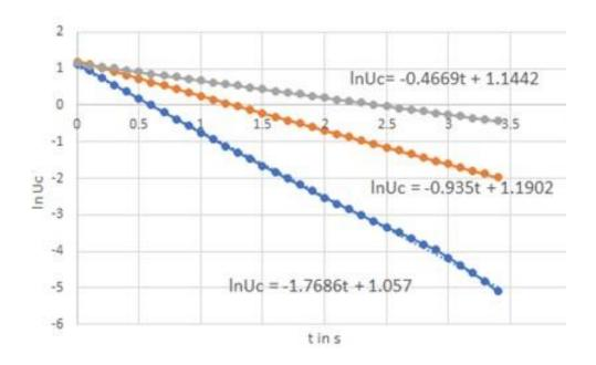
Figure 3: Plotted values of the natural logarithm of the voltage across two identical capacitors connected in series (blue) and parallel (grey) displayed for one single capacitor of capacitance  $10\mu F$ .
