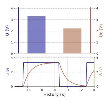
*Figure 2:* Charging and discharging characteristic of a capacitor  $U_C(t)$  controlled by the square waveform voltage U(t) generated by an LDR connected to the GPIO-Pins of the Raspberry Pi
