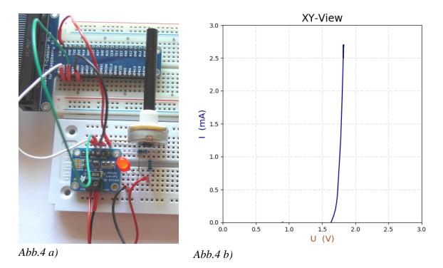
**Figure 4:** a) Circuit board layout with INA219 sensor and Raspberry Pi to record the currentvoltage characteristic I(U) of a light-emitting diode; b) Real-time xy-displayed characteristic I(U) on the graphical interface phypi.py of the PhyPiDAQ-program
