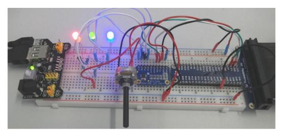
*Figure 5:* Breadboard layout with ADS1115 and three different LEDs for recording their current-voltage characteristic I(U) at the same time.
