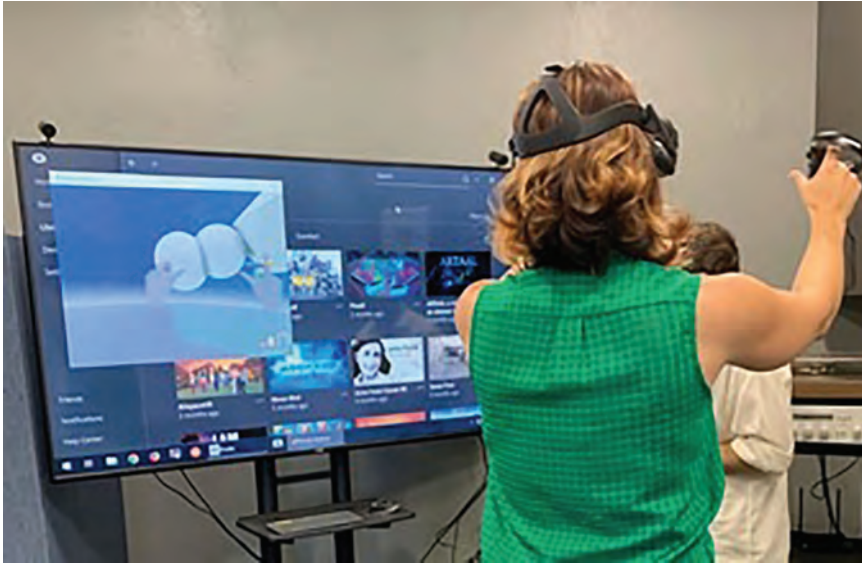
Figure 1. A demonstration of using the Oculus Rift HMD in the XR space. The user is utilizing the Oculus Medium app (the VR sculpting app used in this project), and the computer screen behind them is displaying the HMD view.
