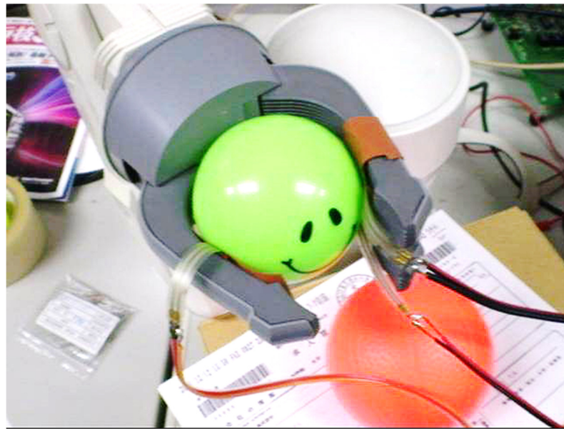
(a) The robot demonstrates a grasp force control of a green softball
