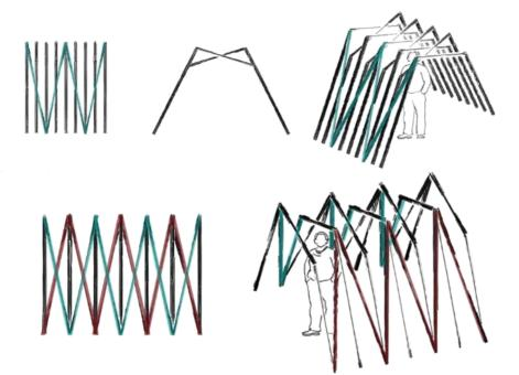
*Figure 27, 28: Second Step: Using V-Bracing in Both Side of Pavilion for Lateral Stability and Retract and Deploy in Horizontal Axis.*
