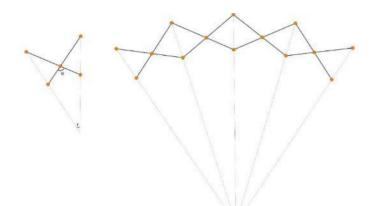
Figure 12: Polar Unit and Linkage in a Close and Open Deployment Position.
