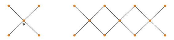
Figure 9: Plane Translational Unit and the Composed Lazy-Tong Scissors Mechanism
