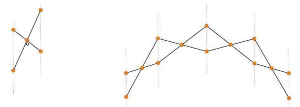
Figure 10: Curved Translational Unit and Linkage
