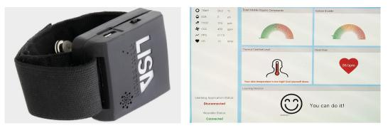
**Figure 2:** The left image shows the LISA wristband, the right image the SmartMonitor app that is connected to the wristband via Bluetooth and that records the physiological data during the training sessions.
