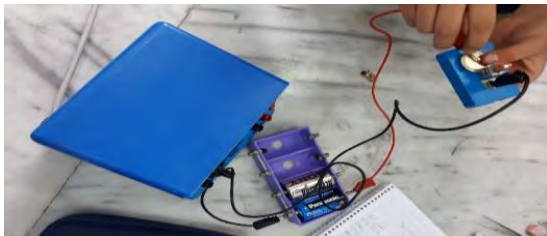
Photograph 4. Conductivity Test of a Coin
