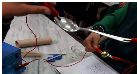
Photograph 3. Testing the Conductivity of a Spoon
