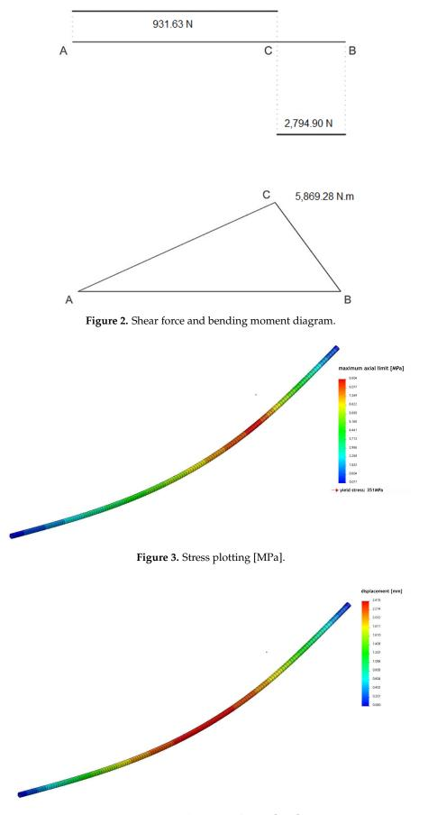
Figure 4. Displacement plotting [mm].
