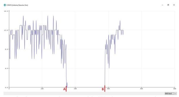
Figure 6. Graph representing the intensity of the UV radiation over time, with point A being the moment when the sunglasses were placed in front of the sensor and point B the moment when sunglasses were removed.
