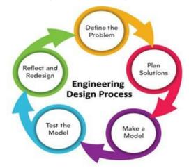
Figure 1. Preschool EFK-Engineering design process model
