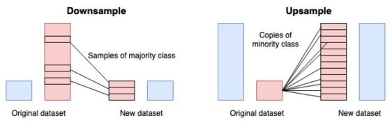
Figure 1. Downsample flow (left) and Upsample flow (right).
