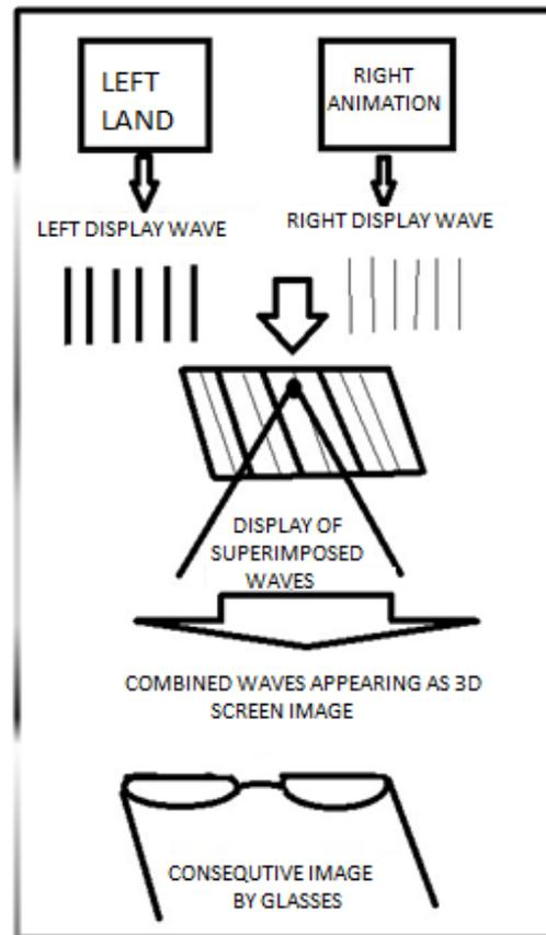
Figure 1. Simple 3D Simulation Image Creation Scheme.
