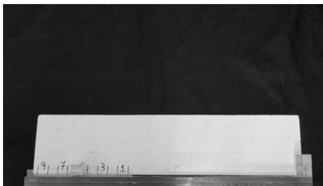
*Figure 1.* The apparatus constructed for investigating length perception with canes as observed from the experimenter's side. To the left side of the apparatus, there is a ruler of acrylic with openings for adjusting each one of the nine stimuli lengths, from one (35 cm) to nine (51 cm). The moveable support is set at the standard stimulus of five (43 cm).
