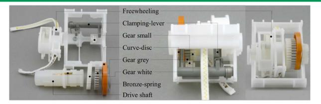
Figure 1. Components of the sun-blind turning unit with one disassembled unit (left) and one assembled unit (right)
